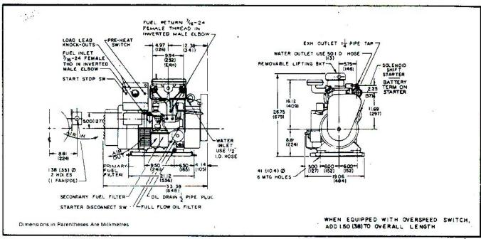
Approx net weights: Raw Water Cooled 500-lb (227 kg). Heat Exchanger Cooled 520-lb (236 kg). Operation Angle—30° in all directions. Onan Sound Shield overall dimensions: L—39.06-in (992.12 mm), W—23.56-in (598.8 mm), H—28.5-in (723.9 mm); approx net weight: 77-lb (34.9 kg).
